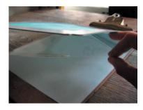
**Step 3:** Pull registration film flat and tight then tape it down to your board/table surface. You can now print onto the film.
