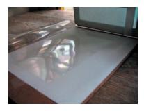
**Step 2:** Take your clear film and tape along one left, right or bottom edge so that you can flip it easily in and out from under your screen. The film is taped on the left edge in the photo above. This becomes your registration guide.
